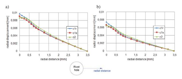
Fig. 9. Radial displacement values vs. radial distance in the upper sheet: a) pressure b) unloading
