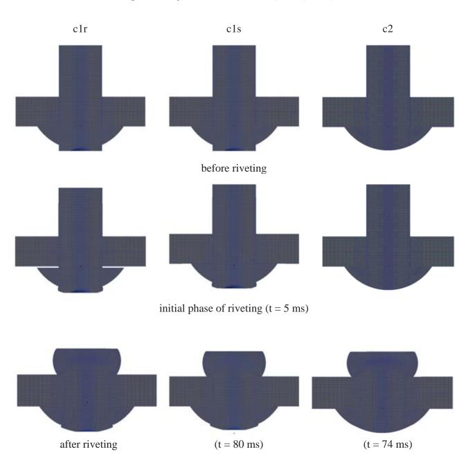
Fig. 5. Rivet deformation
