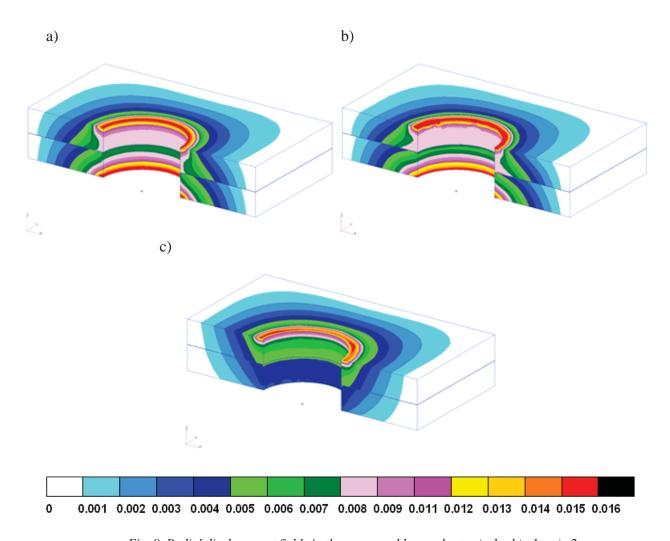
Fig. 8. Radial displacement fields in the upper and lower sheet: a) c1s; b) c1r; c) c2
