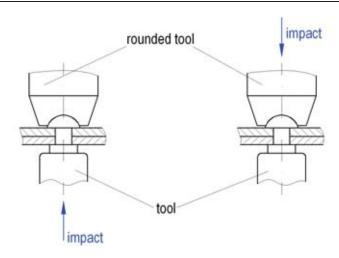
Fig. 1. Manual dynamic riveting process: a) reverse riveting procedure; b) standard riveting procedure
