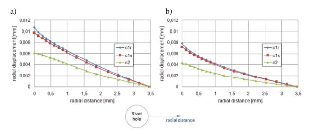
Fig. 10. Radial displacement values vs. radial distance in the lower sheet: a) pressure b) unloading
