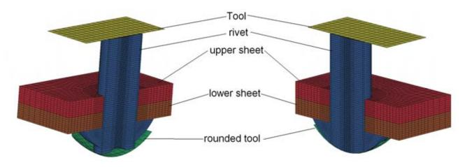
Fig. 2. Model of riveted specimen
